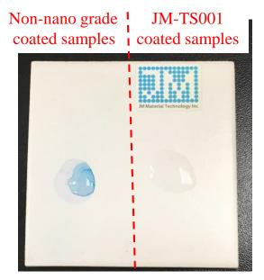
Comparison of methylene blue degradation test. Before UVC light activation(above) and after UVC light activation (right).
