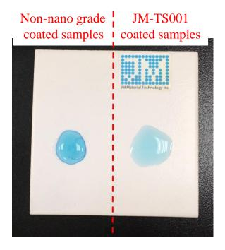
Dye Solution (Methylene Blue) Degradation Test: Drop 1ml of 5ppm Methylene blue solution on each coated surfaces then activate with UVC light for 7 minutes.
